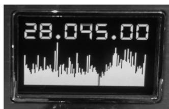
To control the amplitude of the graph in the scan, use the RF-GAIN switch on your equipment.
