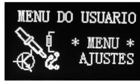
In the menu settings we have the ability to adjust 9 items. These items are basic system settings, such as changing the user name , the number of the desired beep, the time interval between PTT and beep, Anatel Table On/Off, Frequency Meter On/Off in channel mode, Unify or not unify the tuner tuning, control screen brightness, Limit time in carrier seconds, align transverter.
