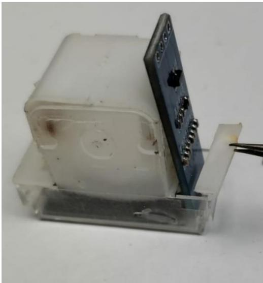
Now you can attach the I2C buss wires to from the Arduino controller to the display...Gnd, Vcc, Scl and Sdk as in the circuit diagram.
